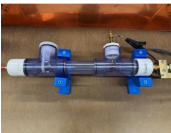
FIG. 12. An image of the physical EA. Some additional EA components included in this image include plastic ring holder for attenuator material (inside left PVC T-junction), broadened anode (inside right PVC T-junction), and clear PVC for qualitative investigation of electron beam behavior.
